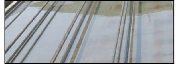
**W**ith Bethlehem's technologically advanced precast concrete construction, your possibilities are endless. Precast is concrete poured into forms in a specialized production facility and hardened in an environment which is carefully controlled to ensure quality. After curing, it is transported to the sight and placed in position.
